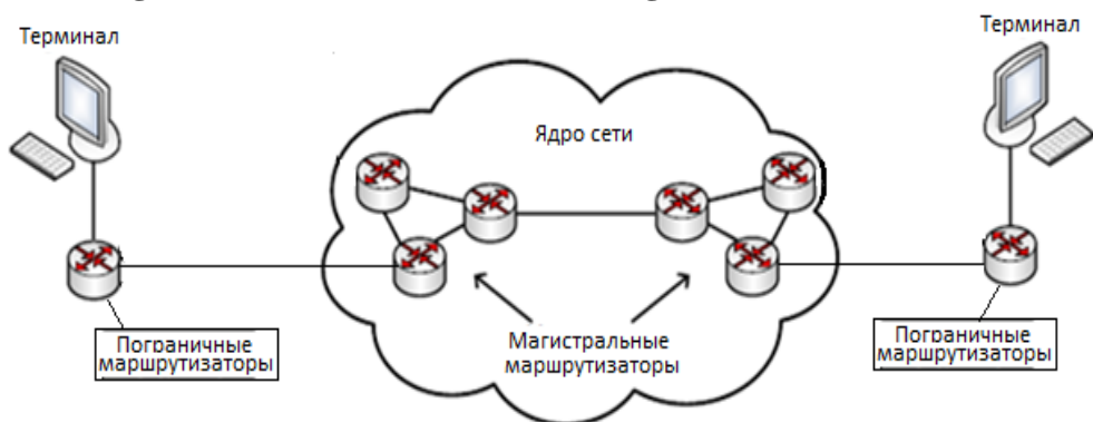
Рис. 2 Сеть, построенная согласно модели DiffServ Figure 2 The network built according to the model DiffServ
