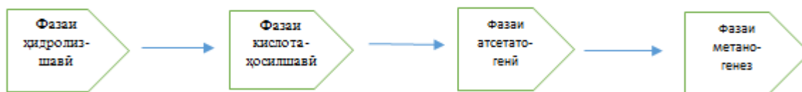
Figure 1. Biotechnological process of biogas production based on natural compounds in household waste
