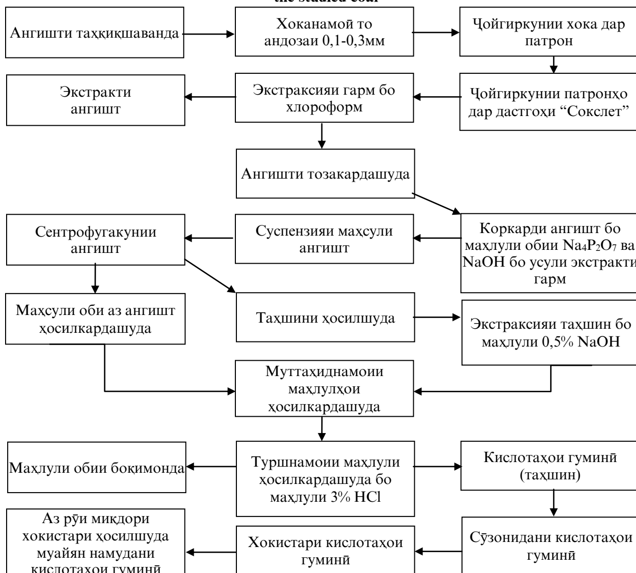
Figure 1. Technique and technology for determining the amount of humic acids in the composition of the studied coal
