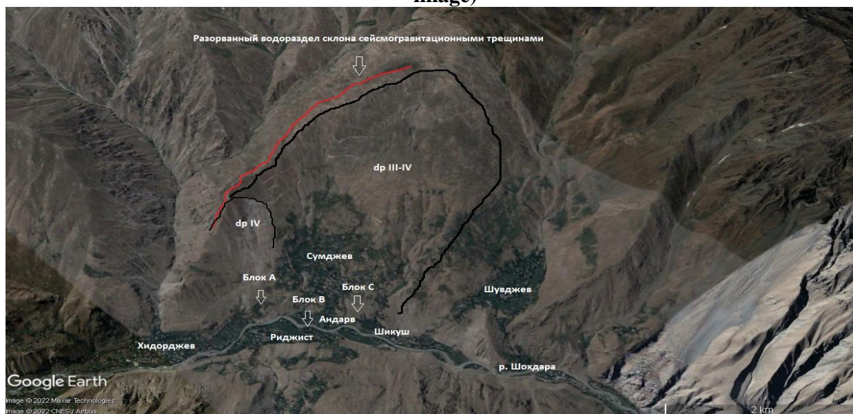
Fig. 3. Overview of the Sumdzhevsky landslide slope. The arrows indicate the locations of the alleged active landslide blocks (A; B; C) according to the developed scenario (from the Google image)
