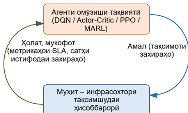
Figure 5. General scheme for adaptive management of computing resources based on reinforcement learning methods
